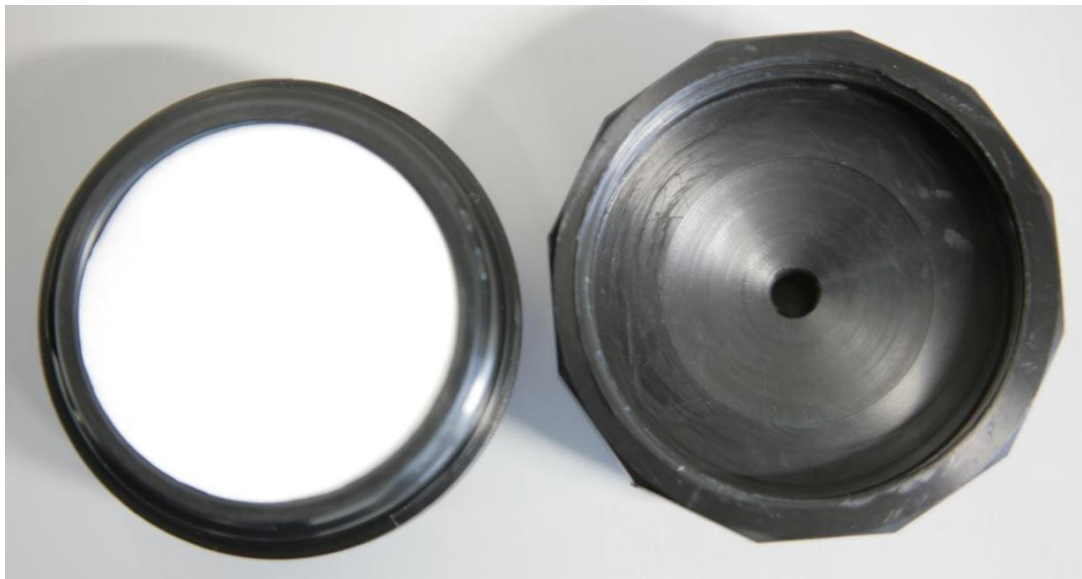
Filter Unit (open, with filter disc and O-seal)
